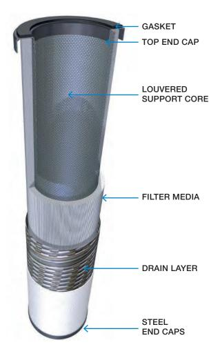
Jonell Systems coalescing elements are available in various standard and custom sizes, pleated and depth configurations to fit virtually every application.
